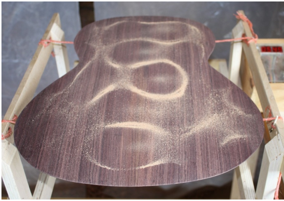
Long 5-pole in Rosewood: 2.0mm/200g – 549Hz
